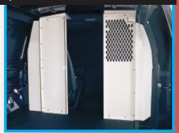
Single panels are available for the driver or passenger side or both. Used together, they leave a walk through.
