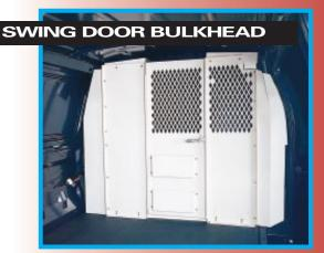
Swing Door Bulkheads provide easy walkthrough access to the rear cargo area.
