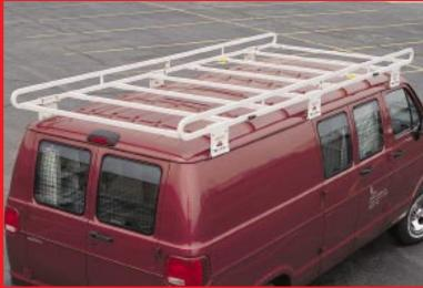
Above: Model 210-3 Safari Rack adjustable center mounting leg with bolt on gutter clamp.
