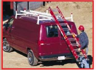
Above: Model 240-3 Ladder Guide installed on a Model 209-3 Aluminum All-Purpose rack and a full size van.
