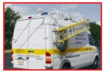
Model 280 EZ-GLIDE™ SYSTEM Rack mounted on Sprinter van with rear slide down system.
