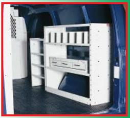
Above: Flat Shelf Unit and Rack Unit installed in a full size van. Also shown are accessory Flat Shelf Bin Dividers, a Retainer Lip and a Drawer Unit.
