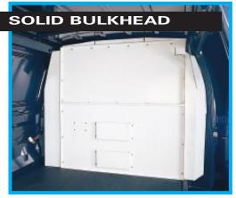
Solid Bulkheads offer the driver maximum protection from shifting loads.
